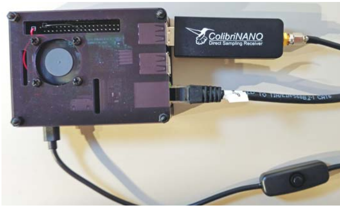
Figure 3 — The ColibriNANO and Raspberry Pi 3 set up for remote server operation.
