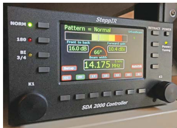
Figure 7 — The optional SDA 2000 controller offers many additional features compared to the standard SDA 100.
