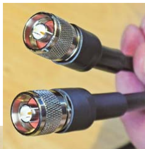
Figure 3 — The type-N connectors installed on the LMR400 with the heat shrink (after all the tests were completed).
