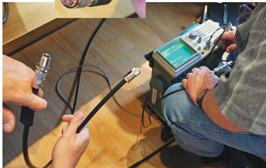
Figure 4 — Claude, VE2BUB, sweeping the cable for any problems.
