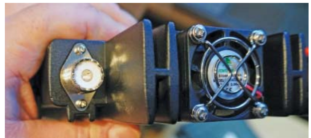
Figure 2 — (Left) On the rear panel, the GPS antenna connects to the SMA connector and two 1/8-inch external speaker jacks are under a rubber cap. (Above) The AT-D578UVIIIPRO uses a single SO-239 antenna jack. The radio has a triplexer built in, and the user will need to supply a suitable multiband antenna.
